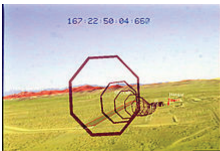
LandForm video map overlay marking runways, road, and buildings during 1999 helicopter flight test.
